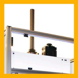
Offers 20" of stroke, and up to 4000 lbs of force for your assembly application.
